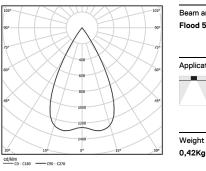
Beam angle Flood 56° Application Weight
