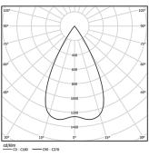
Beam angle Flood 56° Application Weight 0,42Kg
