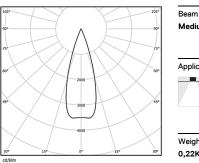
Beam angle Medium 31° Application Weight 0,22Kg
